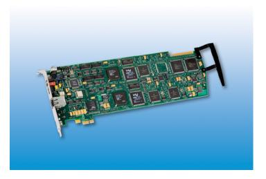
technology and they are well-suited for server-based CT systems under Windows and Linux. They also provide a powerful platform for creating sophisticated Interactive Voice Response (IVR) applications for the small and medium-sized enterprise market segment. Features such as fax and software-based speech recognition processing enable unified messaging applications. They also provide Automatic Gain Control (AGC), so even a weak telephone signal can be recorded and replayed with clarity.
