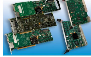
tone detection/generation, echo cancellation, and voice compression, as well as trunking, fax, conferencing, and VoIP functions in a single PCI, CompactPCI, or PCI Express slot. The universal port feature eliminates the need to use multiple specialized boards, provides easy access to all supported features, and significantly reduces the time spent on configuration and development.
